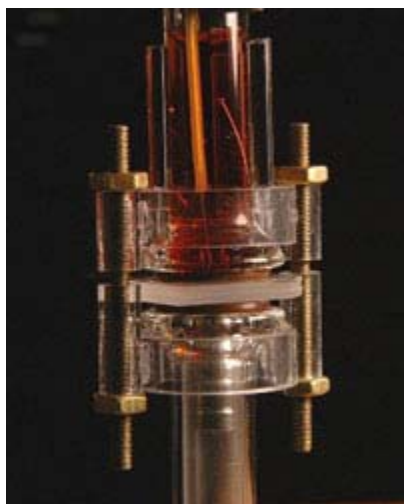
A low energy nuclear reaction cell used this year at the University of California, Berkeley, US, in an attempt to replicate research conducted at the US Space and Naval Warfare Systems Center, San Diego
